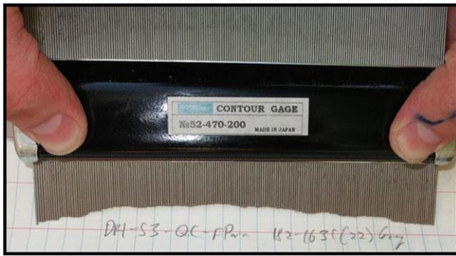
**Figure 4.** Contour gage photographed after being pressed perpendicularly against the bedrock surface. Photographs were processed using image analysis to determine surface roughness, calculated as the standard deviation of pin heights. [Colour figure can be viewed at [wileyonlinelibrary.com](http://wileyonlinelibrary.com)]
